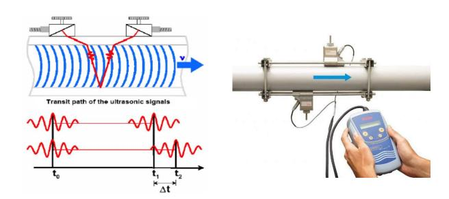
The two transducers are used alternately as an emitter and receiver: the difference between the sound and the flowing fluid velocities creates a small time difference between upstream and downstream sound transmissions.
