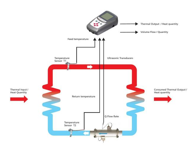
Equipped with clamp-on flow sensors and two non-intrusive surface T probes, the Ultraflux clamp-on flowmeter functions as a BTU meter and measures and displays the two temperatures (inlet and outlet), their difference and compute the energy flow from the raw flow rate and the characteristics of the fluid. Actual Energy flow (delivered or exchanged) is displayed in kW and Energy is totalized in kWh.
