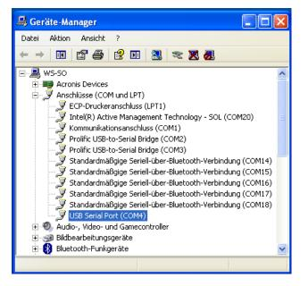
COMx set must be between COM1....COM9 and it should be ensured that there is no double occupancy of the interfaces.
