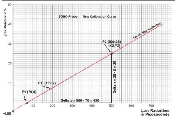
The coefficient m1 is calculated from the slope of the curve Cal14:
