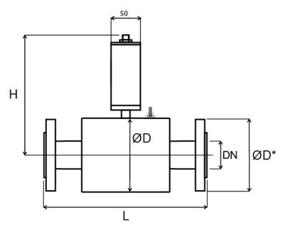
$D^*$  ... The outside diameter corresponds to the required pressure class and standards.
