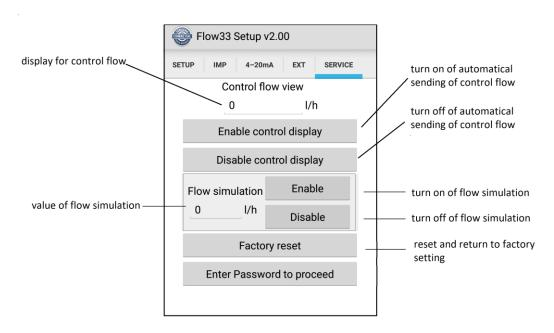
For termination of the communication, always perform "DISCONNECT" to disconnect from the meter on SETUP tab. In case of an unexpected error, for example, failure to reconnect to the meter, possibly in case of "frozen" connection, restart the meter by a short disconnection from power.
