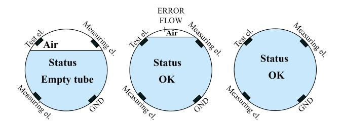
Installation in piping and placement of measuring electrodes in flow sensor
