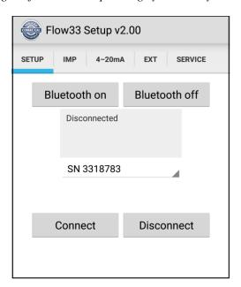
Installation takes its course in a classical manner according to the device used. After installation and launching the program, the user has individual tabs (see figure) according to associated individual parameter groups. Prior to connecting and setting, it is necessary to pair both devices in Bluetooth setup right in the device (except for FLOW 33 Setup software).
